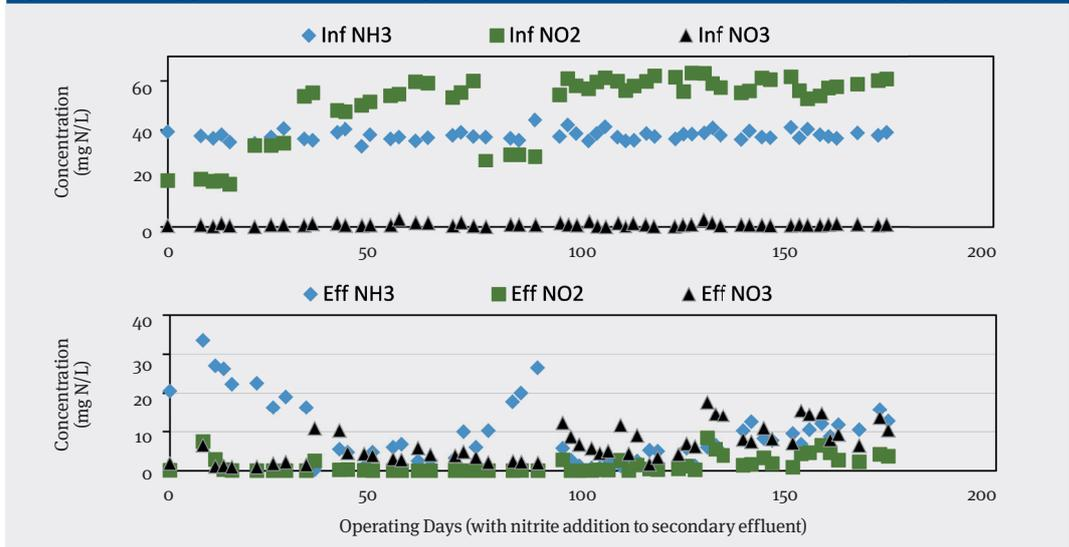
provided with sufficient oxygen to support nitrification, the research team hypothesized that deammonification may have been occurring within the BBF biofilm or granules within the biofilter due to substrate and oxygen diffusion limitations. The pilot was therefore extended to evaluate the feasibility of a mainstream deammonification for sustainable mainstream nitrogen management.
