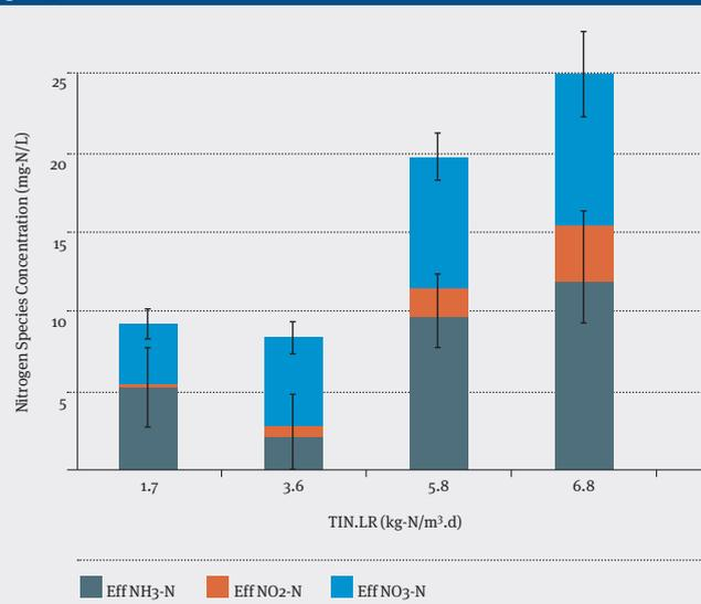
Nitrogen fractions of the AMX BBF effluent in different phases of the pilot study
